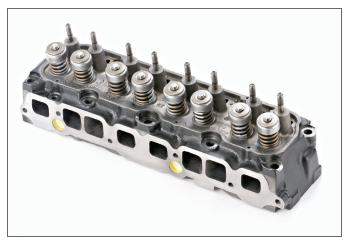
The 8-port version cylinder head casting is used on all versions of the Vortec 3.0L engine. Certain versions of this common casting are machined to accept the MPFI Fuel Injection System.
